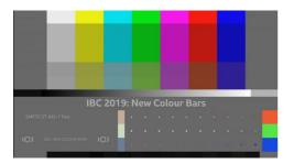
The EBU colour bars will help to measure luminance response and visualize saturation, hue shifts, and near-black performance. It will also have a test for correct Quad-3G-SDI and 2SI installation.
