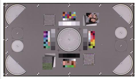
Figure 1. Chart 42 16X9 Version 2 used for resolution tests
