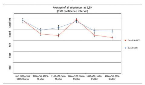
Figure 1. The positive influence of MCFI is reflected in the higher values of the blue points compared to the red ones. The improvement that can be obtained seems to be larger for material with a 50% shutter, which makes sense as these shuttered images can be expected to be sharper (with less motion blur), and thus better suited to calculate new frames from.
