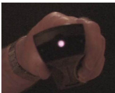
Figure 13: Infra red output of a remote control
