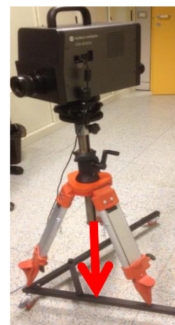
CS 2000 spectroradiometer on wheeled tripod with led laser to measure height
