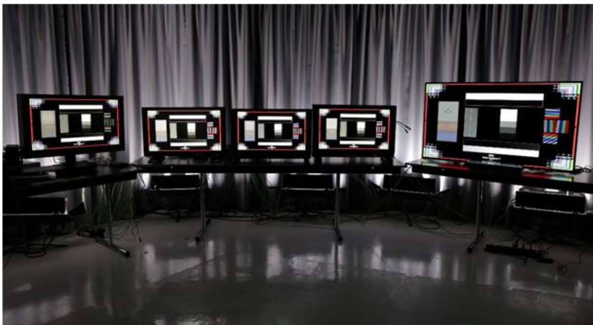
Figure 1: Impression of the studio set-up showing five displays outside the ‘black box’. Mid-grey backdrop curtains were lit by D65 illumination to assist the subjective quality evaluation.
