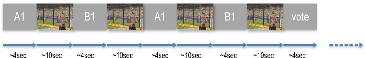
Figure 5: Illustration of the time sequential approach of the DSCQS method. Note the number is used to indicate which assessment unit is being scored.
